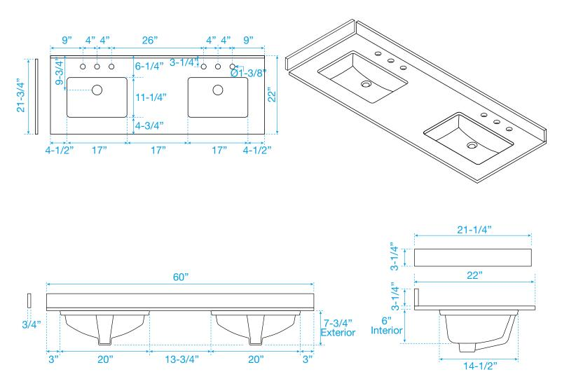
Note: Side splash is reversible. Due to high probability of breakage, the backsplash comes in two pieces, cut from the same piece. All measurements are  $\pm$  1/4".
