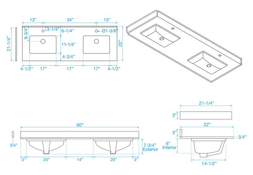
Note: Side splash is reversible. Due to high probability of breakage, the backsplash comes in two pieces, cut from the same piece. All measurements are  $\pm$  1/4".
