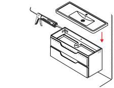
(5) Install the counter. Seal around the top of the cabinet with clear silicone sealant. Do not over apply. Allow to dry for over 24 hours for proper curing.
