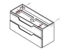
③ Fasten cabinet to wall by attaching screws through the bracket holes, and by attaching the lower brackets. Use a spirit level to ensure vanity is leveled.
