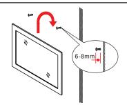
(8) Install the screws into the wall anchors, leaving enough of the screw exposed to hang the mirror - approx. 1/4"-1/2".
