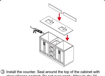
clear silicone sealant. Do not over apply. Allow to dry 24 hours for proper curing.
