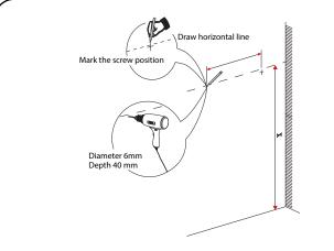
4 Install the mirror: use a pencil to mark the placement of the screw holes on the wall, drill the holes and insert the plastic wall anchors.
