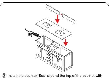
3 Install the counter. Seal around the top of the cabinet with clear silicone sealant. Do not over apply. Allow to dry 24 hours for proper curing.
