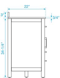
\*Note: Due to high probability of breakage, the backsplash comes in two pieces, cut from the same piece. All measurements are ± 1/4".
