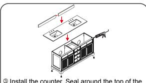
③ Install the counter. Seal around the top of the cabinet with clear silicone sealant. Do not over apply. Allow to dry 24 hours for proper curing.
