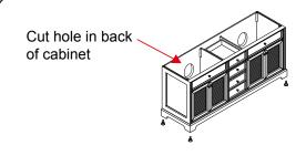
① Installer must cut appropriately sized hole in back of cabinet to accomodate existing placement of hot & cold wall valves & drains.
