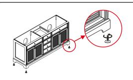
② Adjust the adjustable feet according to the floor.
