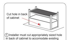
placement of hot & cold wall valves and drains
