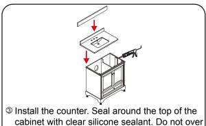
apply. Allow to dry 24 hours for proper curing.
