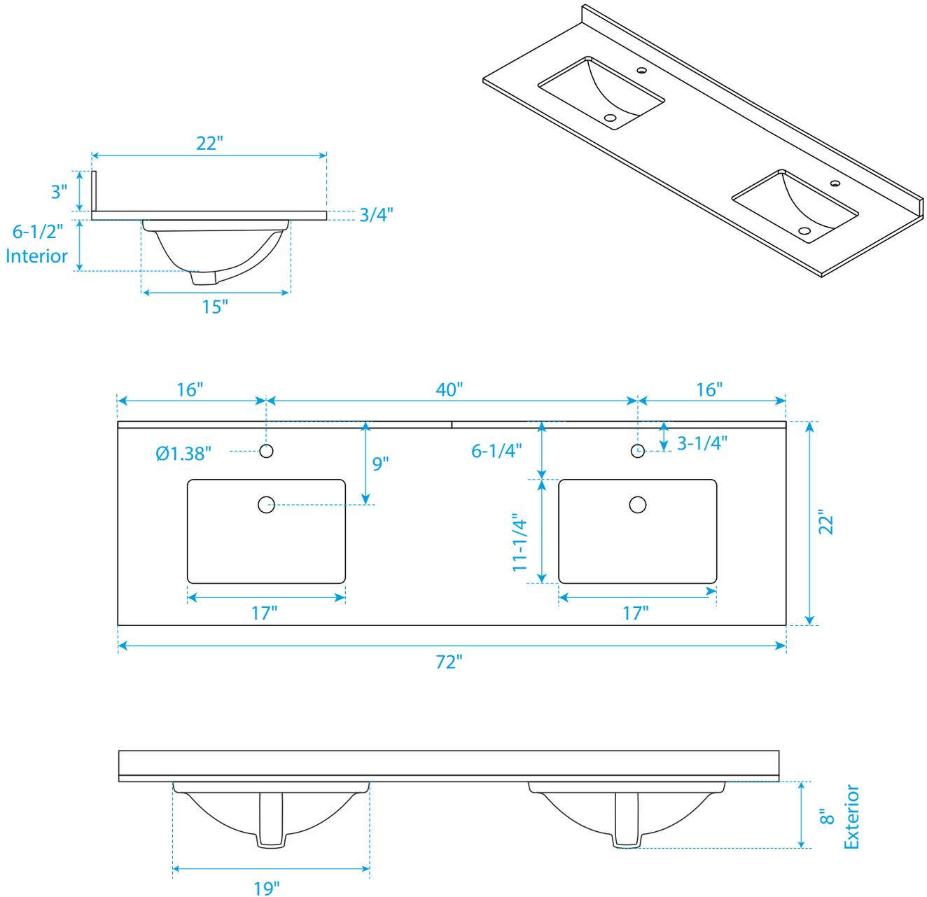
Note: Due to high probability of breakage, the backsplash comes in two pieces, cut from the same piece. All measurements are  $\pm 1/4"$ .
