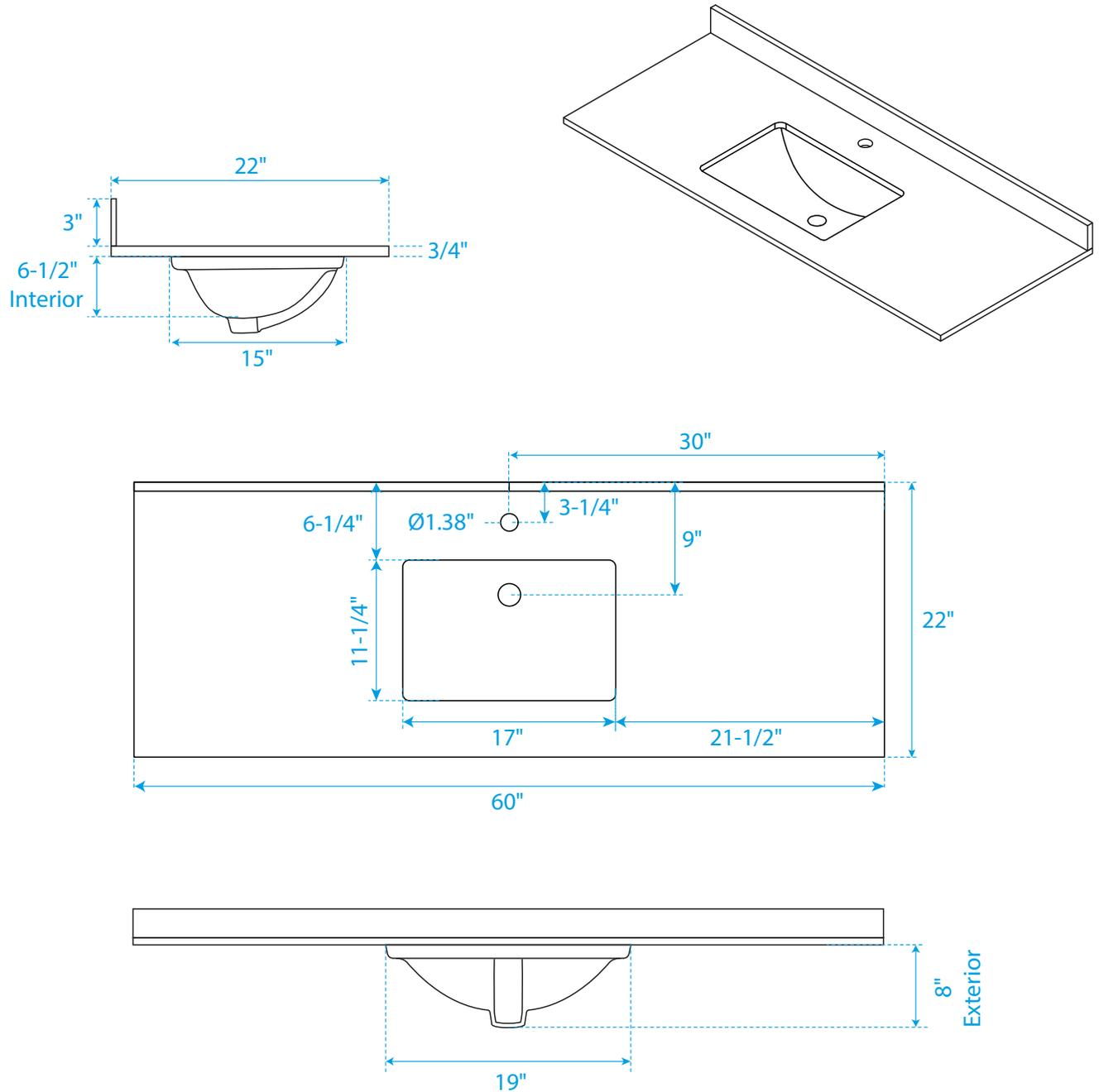
Note: Due to high probability of breakage, the backsplash comes in two pieces, cut from the same piece. All measurements are  $\pm 1/4"$ .
