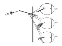
(8) Install the screws into the wall anchors, leaving enough of the screw exposed to hang the mirror - approx. 1/4"-1/2".
