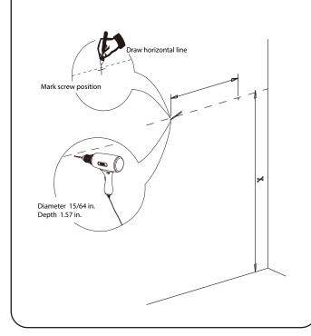
② Attach the bracket by screwing into a wall stud for reinforcement.
