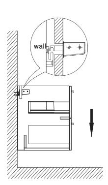
4 Adjust the mounting attachment as required
