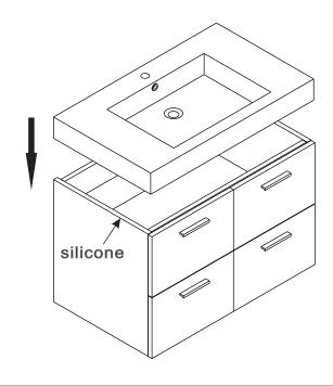
6 Licensed professional installation is recommended. These instructions are for mounting into studs or other in-wall reinforcement, drywall alone is not sufficient to support wall-hung vanities. Other installation techniques may require a licensed professional.
