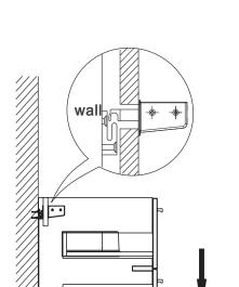
4 Adjust the mounting attachment as required
