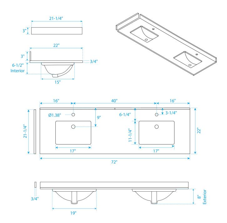
Side splash is reversible. Note: Due to high probability of breakage, the backsplash comes in two pieces, cut from the same piece. All measurements are  $\pm$  1/4".
