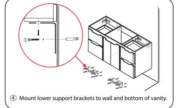
③ Fasten cabinet to wall by attaching screws through the bracket holes, and by attaching the lower brackets. Use a spirit level to ensure vanity is leveled.
