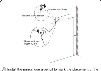
4 Install the mirror: use a pencil to mark the placement of the screw holes on the wall, drill the holes and insert the plastic wall anchors.
