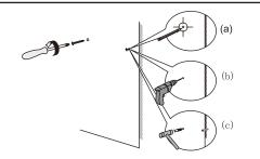
② Install the mirror: a)use a pencil to mark the placement of the screw holes on the wall, b)drill holes, c)insert the plastic wall anchors.
