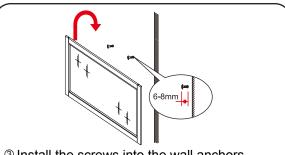
③ Install the screws into the wall anchors, leaving enough of the screw exposed to hang the mirror - approx 1/4" - 1/2".
