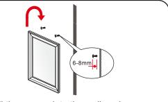
© Install the screws into the wall anchors, leaving enough of the screw exposed to hang the mirror - approx 1/4" - 1/2".
