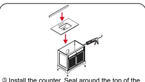
Install the counter. Seal around the top of the cabinet with clear silicone sealant. Do not over apply. Allow to dry 24 hours for proper curing.
